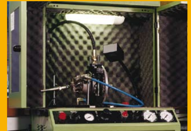
10.6 Vibration Sorting Rig
